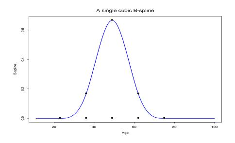
Figure 3: An example of a single cubic spline.
