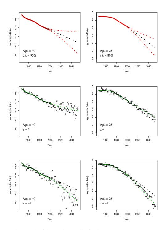
Figure 5: An example of the P-spline model. At the top are cross-sections at ages 40 and 75 of the fitted model, showing the mean projection and the 2.5th and 97.5th percentiles. The second and third graphs show cross-sections at ages 40 and 75 of two independent simulations, one with  $z_i = 1$  and one with  $z_i = -2$ . Circles before 2003 represent added Poisson noise using the actual exposures  $E_{x,t}$  before 2003 and the exposures  $E_{x,2002}$  after 2002.
