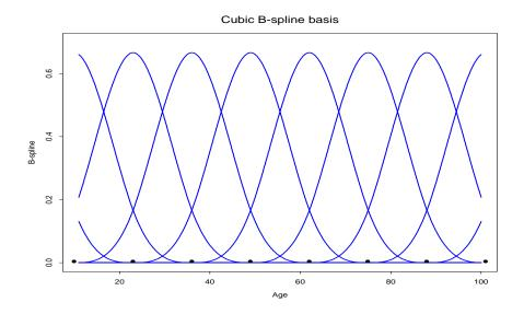
Figure 4: An example of a spline basis made up of cubic splines.
