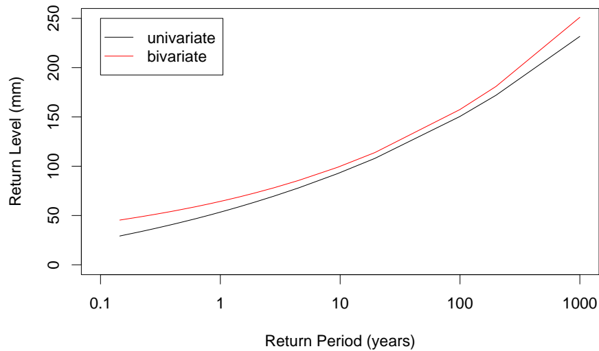
Figure 4.19: Plots of return levels against return period for site 2 based on the informative posterior distribution for the univariate and bivariate models
